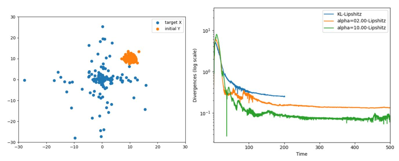
Learning Student - t(0.5) from N((10, 10), I) by Lipschitz regularized GPA with different f. Blue:  $f_{KL}$ , Orange:  $f_{\alpha}$  with  $\alpha = 2$ , Green:  $f_{\alpha}$  with  $\alpha = 10$ .
